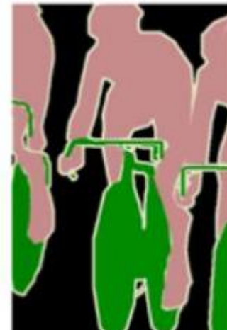
Improved segmentation results with skip connections [LON2015].
