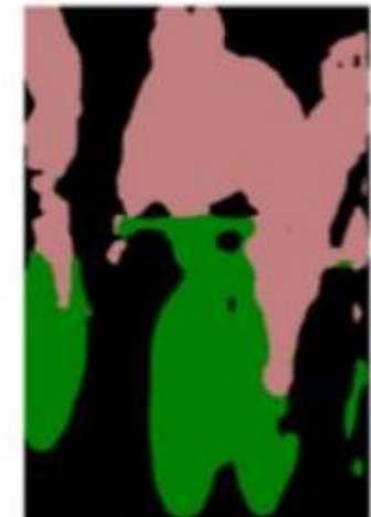
Improved segmentation results with skip connections [LON2015].
