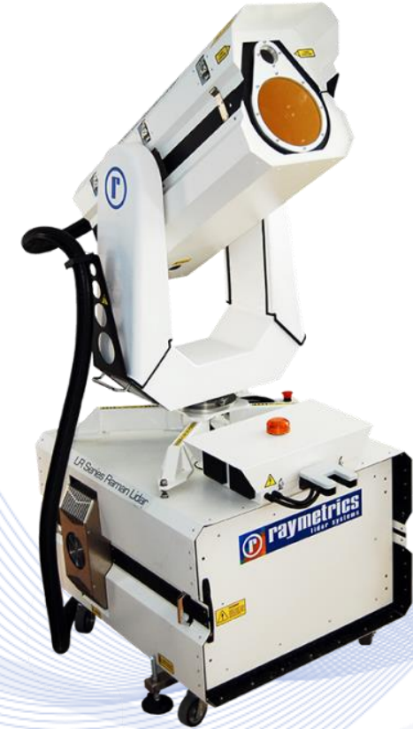
Lidar smoke detector.
