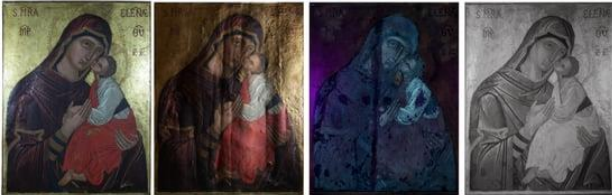
Madonna dell'Elemosina (Biancavilla, Italy). Left to right: diffused visible light; visible grazing light; UV fluorescence; IR reflectography [ARM2021] .
