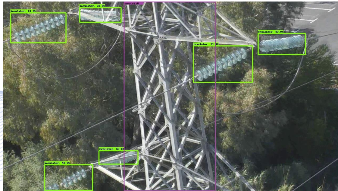
a) Face detection; b) Electrical Insulator detection.
