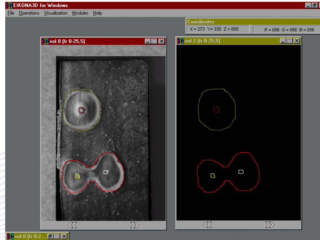
Contour following on a tooth cross-section.
