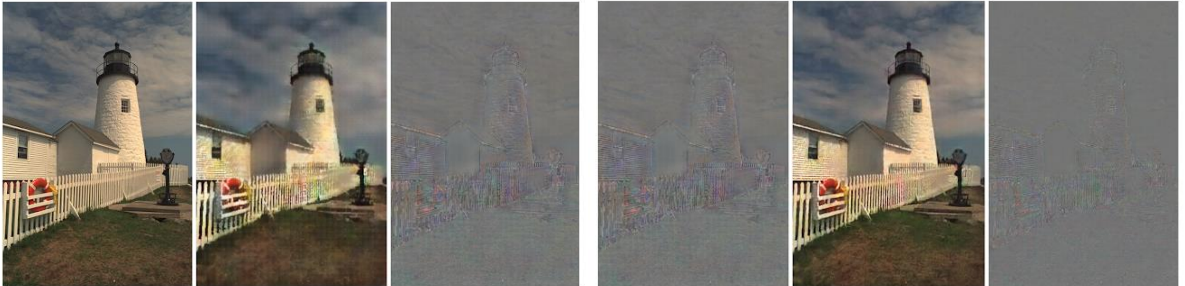
Left: Original image, I = R[0] . Center: Reconstructed image, P[1] . Right: the residual, R[1] , which represents the error introduced by compression.
