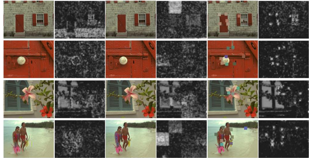
Figure 6: Local quality estimation results on examples of non-global distortion from TID2008. Column 1,3,5 show (a) jpeg transmission errors (b) jpeg2000 transmission errors (c) local blockwise distortion. Column 2,4,6 show the local quality estimation results, where brighter pixels indicate lower quality.
