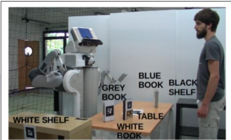
FIGURE 9 | Initial state of the world in the Clean the table scenario. In this task, the robot and the human share the goal of cleaning the table together.
