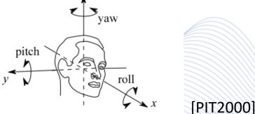
That is why they are also called 6-degree-of-freedom (6-DOF) devices. Gyroscope and motion sensors are also deployed.
