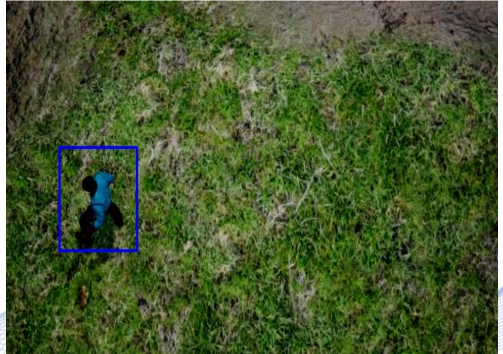
Person detection using YOLO v3.
