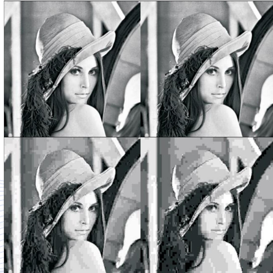
a) Original image; b) 90% JPEG compression quality; c) 5% JPEG compression quality; d) 1% JPEG compression quality.
