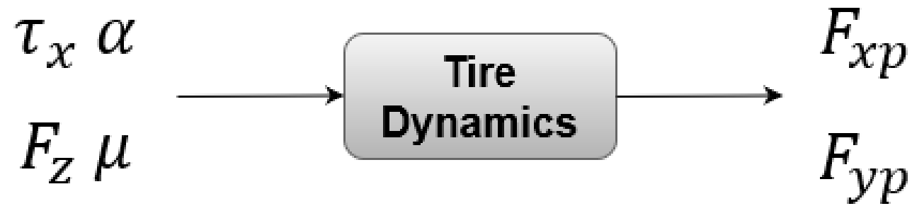
Figure 8: The main concept of the tire dynamics.
