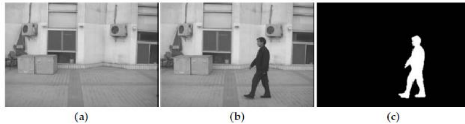
Ex. of Silhouette extraction: a) background image , b) original image, c) the extracted silhouette from the original image.
